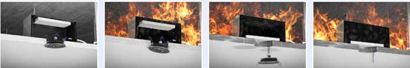
The effect of the heat causes the fire-retardant coating to intumesce, which prevents the fire and smoke from spreading.
