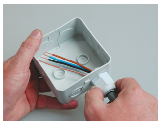
Cable gland M25 Clamping area Ø 11 - 17 mm. Use casting compound only in a dry cable junction box.
