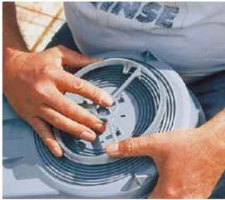
Clip the front ring onto the housing.
