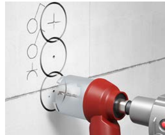
The centring holes created serve as a precise guide for the diamond core bit.
