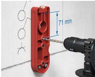
Drill the first centring hole through the guide hole in the drilling template at a distance of 71 mm.
