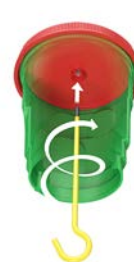
M5 metal nut – secure mounting of light hooks up to 100 N (10 kg) according to DIN EN 60670.
