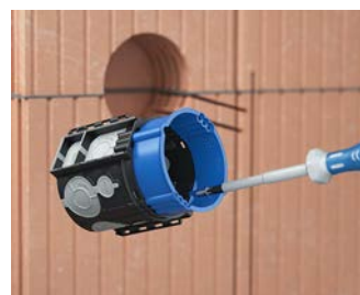
If more installation compartment space is required, the plaster levelling ring can be fitted before inserting the box and aligned according to the planned plaster thickness.
