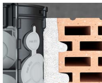
UP 1 ECON ® - Installation with plaster, air-tight
