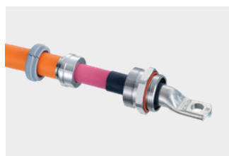
1. Slide cable lug through
