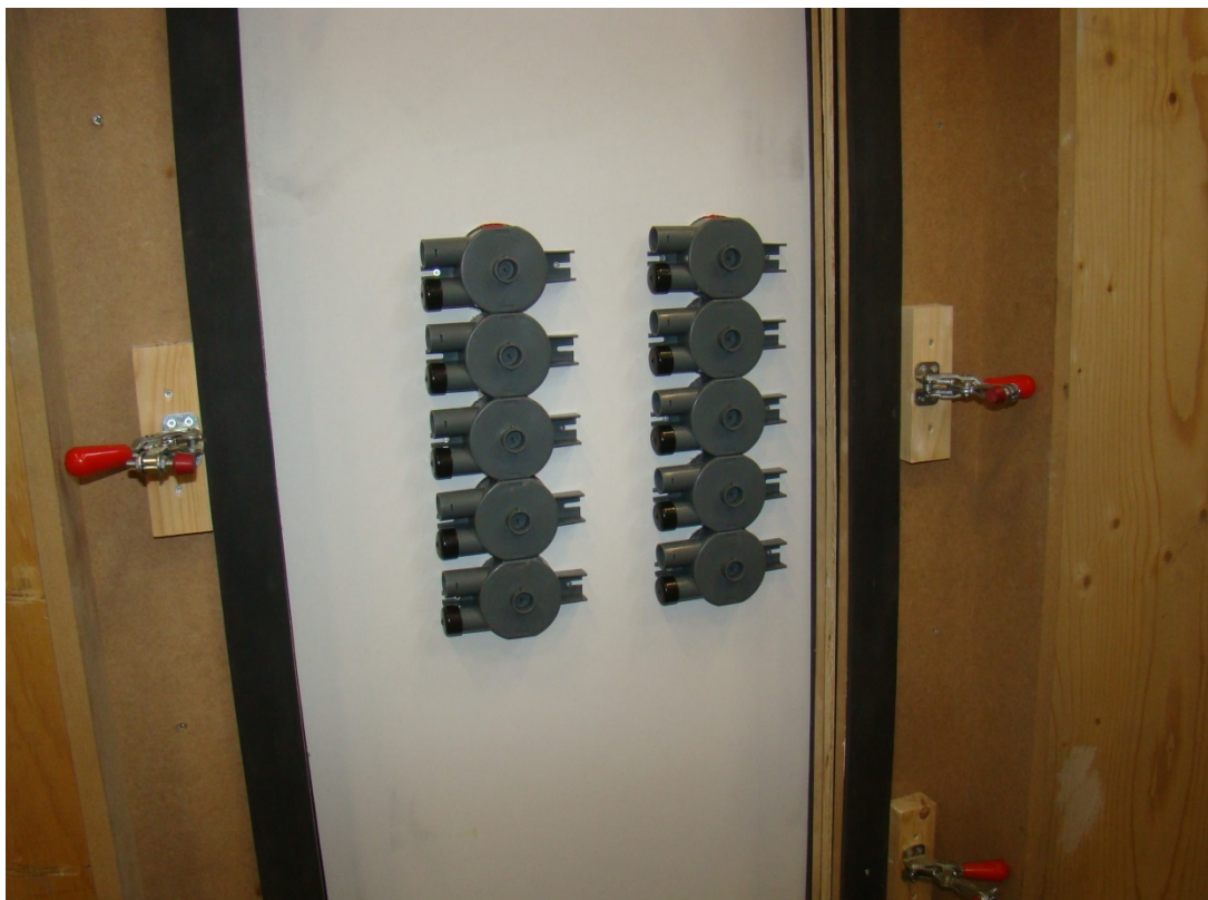
Picture B.2 S_a test, back side panel fixed at pressure cabinet side, capped boxes
